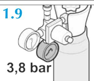
The **minimum working** pressure of the Distributor is **3,8 bars**. Afterwhich the **CO<sub>2</sub>** cylinder needs to be substituted.
